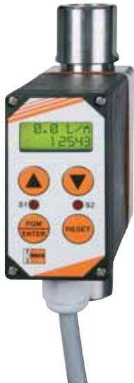
The evaluation unit changes the frequency signal of the pickup into a 3(4)-digit flow reading with selectable measurement unit (top display line), and into a scalable analogue signal. The flow quantity is added up in a part quantity meter and a total quantity meter and then displayed in the bottom line of the screen. The quantity meter's units of measurement are selectable.
