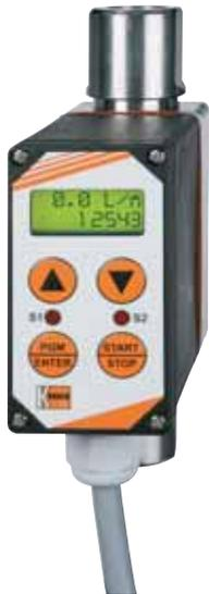
The evaluation unit changes the frequency signal of the pickup into a 3(4)-digit flow reading with adjustable scale (top line of display), and a scalable analogue signal. The dosage is displayed in the bottom line of the display. The unit of measurement can be selected. Included are two relays with floated output changeover contacts for various functions. The relay (S1) can be used to execute the flow monitoring, total volume monitoring, fine dosage or the pump control.
