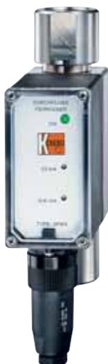
The DF-...MA evaluating electronics converts the frequency signal from the measuring sensor to a 0(4) -20 mA, 0-10 V<sub>DC</sub> analogue signal. It is ideally suited for precise teletransmission of flow-rate measurements for indicating devices, recorders or controllers, for example.
