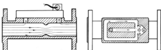
The bypass channel contains the oscillator – the measuring cell itself. When the medium flows through the measuring cell, a liquid column oscillates in a U-shaped channel mounted to the left and right. This oscillation frequency is proportional to the flow velocity.
