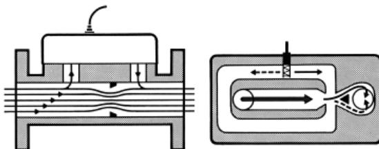
The bypass channel contains the Oscillator – the measuring cell itself. When the gas flows through the measuring cell, a gas column oscillates in a U-shaped channel mounted to the left and right. This oscillation frequency is proportional to the flow velocity and thus to the total volume flow. The oscillation frequency is sensed with a hot wire sensor. An electrical alternating signal is generated that is displayed in the seriesconnected electronics.
