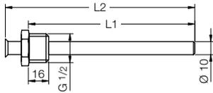
Thermowells 1/2 NPT, internal Ø 8 mm
